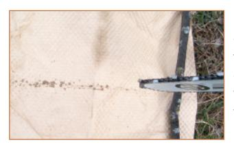
Repeat this process until there is a fine spray of oil on the paper. If you have more splatter than shown in the picture at left, turn the dial clockwise in small increments to close the valve. When you have achieved the correct flow, tighten the set screw and replace the motor housing cover.
