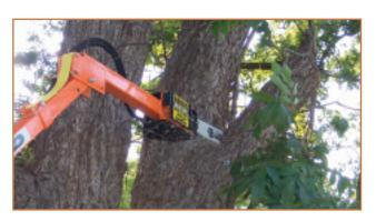
When beginning a cut, position the saw on a branch and lower your loader until you see slack in the yellow strap. This means that the required weight of the saw is resting on the limb to make a clean cut. Do not lower your loader to assist in making the cut. The weight of the saw is all that is required to make each
