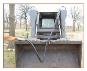
The saw is now shown in the transport position. When driving to and from your work site, always keep the saw folded and pinned to protect it from the wear and tear that bouncing can cause. Always be aware of power lines and other hazards that may be hanging in your path.
