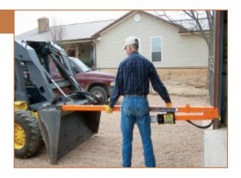
Every tractor has its hydraulic hookups in a different location. For this reason, your Limbinator Saw does not include the hydraulic lines that attach to the tractor. You will need to purchase these lines with a minimum of 3/8" hydraulic hose. Measure from the auxiliary hookups of your tractor to the hydraulic hookups on your saw. Allow enough slack in your lines for the full rotation of your bucket. This skidloader has 6.5' of hydraulic line.
