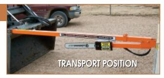
may damage pins and the yellow nylon strap. Use caution when driving under power lines and low hanging branches. Adjust the height of your saw by raising and lowering your loader to clear obstacles that could potentially get caught on your saw during transport.
